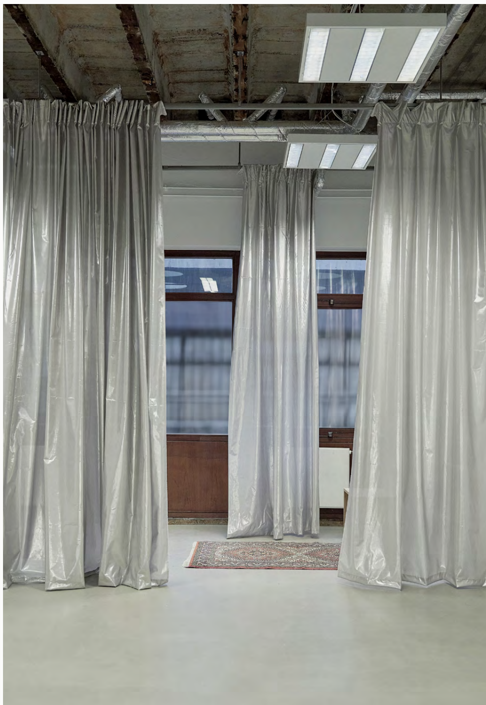
8.2 Changing Room Custom ceiling hanging structure from stainless steel, silver Thermo fabric for curtains. Planned as changing rooms, the curtains made from technical thermo fabric can be moved on a costume suspended rail. Making it possible to create multiple spacial situations, revealing the windows behind or being pushed away completely. Composed of freshly build, found and restored items.
